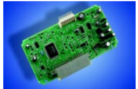
HVAC Control Assembly
