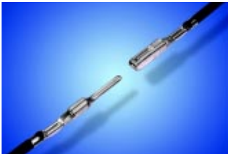
MX150™ Terminals 14,16,18, 20 AWG Tin Plated Female 33012, Male 33000 Gold Plated Female 33001, Male 33011
